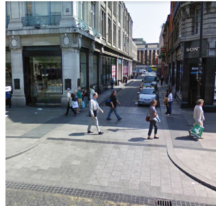
Raised table crossing along O'Connell Street
